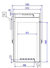
Drain Electrical inlet (power) RO Refrigerant Outlet
